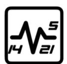
**FREQUENCY.** Switch through the different frequencies with the  $\blacktriangle/$ -buttons. With 5 kHz you will only be able to find big objects very deep in the ground and miss for example small jewelry nearer to the surface. With 21 kHz you will be able to find that small jewelry exceptionally well but aren't able to search very deep. The frequency is set to 14 kHz by default, which is optimized for most conditions and is ideal for most detectorists.
