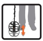
**GROUND BALANCING**. For automatic Ground Balancing, hold the lower ■-button and pump the coil up and down from about 20 cm down close to the ground, until you hear a confirmation sound. You can manually ground balance by using the ▲/▼-buttons after pressing the lower ■-button once.
