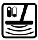
**GROUND TRACKING**. Press and hold the lower -button and press the -button to activate or deactivate the Ground Tracking function. The detector will calibrate to the ground automatically to reduce false signals caused by mineralization.
